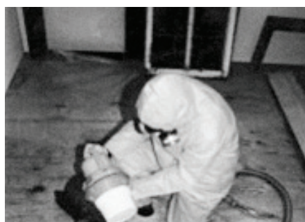
e) Wash/Replace Coarse Prefilters if Necessary
