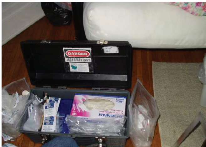
FIGURE 5.11a Dust sampling equipment.
